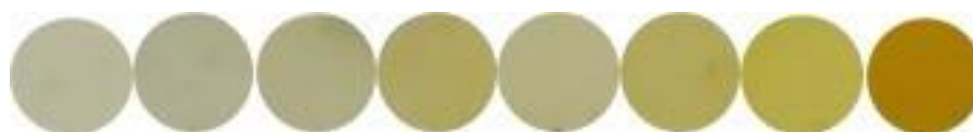
Figure 2. Sensory colorimetric films after dipping in 10 ml of honey solutions for 2 hours at room temperature.
