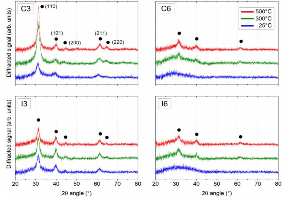
Films deposited at higher pressure require annealing at 500°C to achieve crystallization
