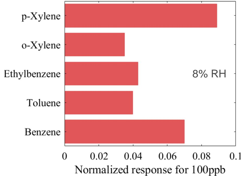
Cross-sensitivity tests with I6 for BTEX showed great sensitivity for all compounds with an enhanced response for para-Xylene
