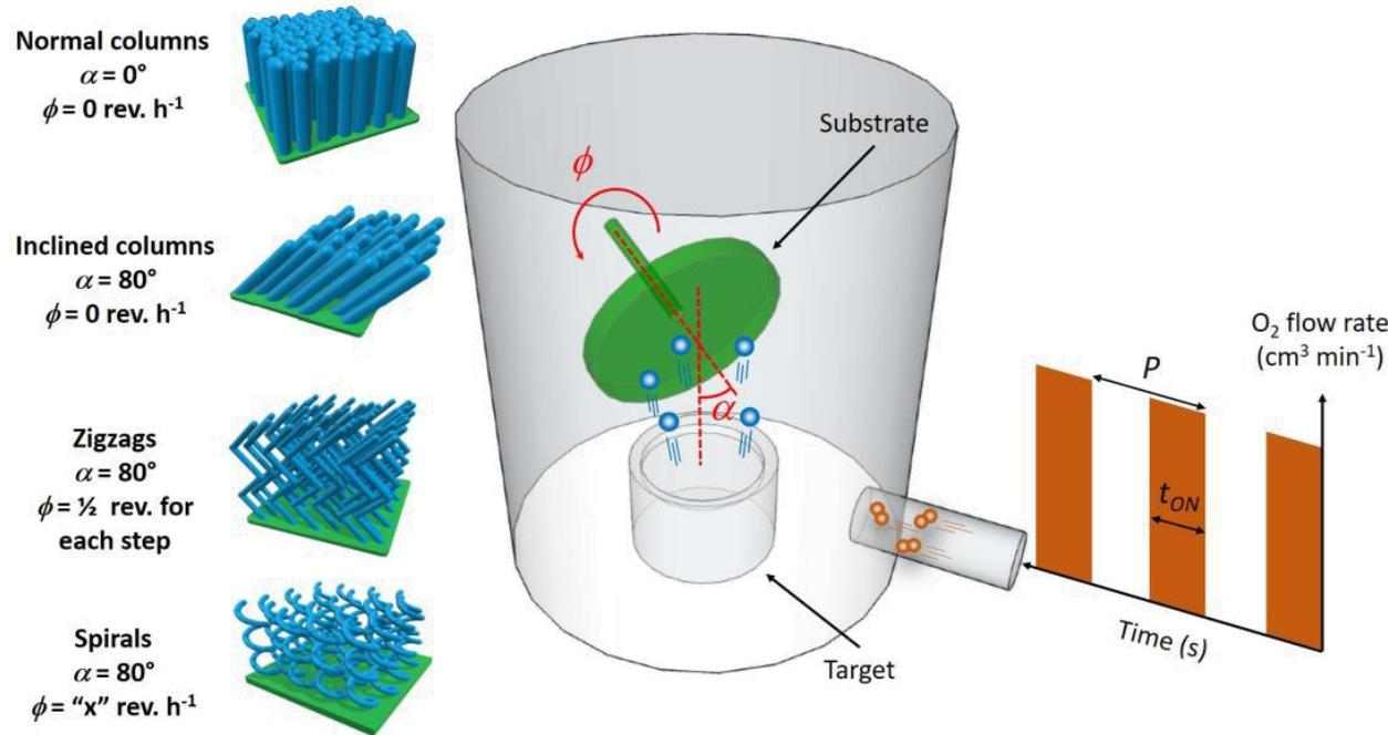
Two parameters were studied, 4 films deposited with a thickness around a thickness of 250nm, and a constant power and oxygen flow :
