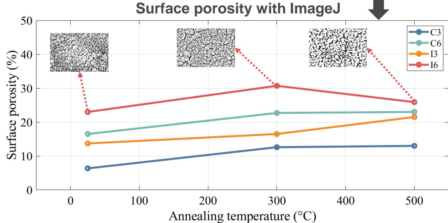
Tilted depositions & higher deposition pressures were found to increase the bulk and surface porosity resulting in higher surface areas
