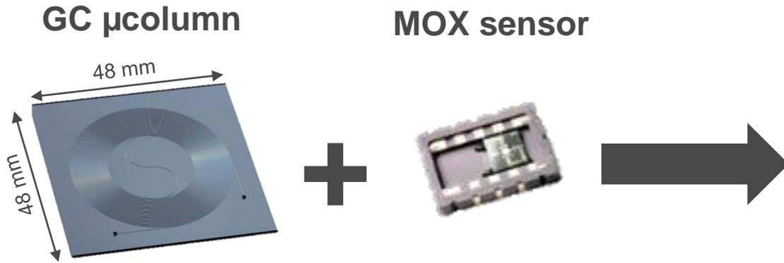
By adding a GC micro-column in front of the MOX sensor, we are able to selectively detect BTEX compounds in a mixture, and under high relative humidity values (60%).
