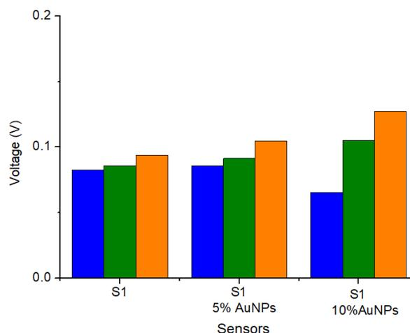
**Figure 1.** Sensors response to glucose at increasing concentrations (blue= $10^{-4}$ M; green= $10^{-3}$  M and orange= $10^{-2}$  M) depending in the percentage of AuNPs applied in the membrane matrix. .
