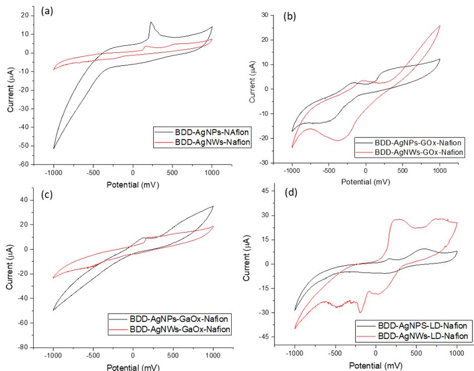
**Figure 1.** Electrochemical response of the sensors of AgNPs bioET (black) and AgNWs bioET (red) in a 50% diluted Classical Whole Milk in 0.1 M KCl solution.
