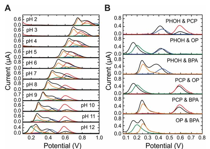
Fig. 4. Baseline corrected square wave voltammograms obtained after A) pH screening (pH 2 to 12) in BR buffer of complex mixture (black line) using 10  $\mu\text{M}$  concentration of each phenol (1:1:1:1 ratio) and B) binary mixture of phenols (black line) of 10  $\mu\text{M}$  concentration of each phenol (1:1 ratio) in pH 12. Single phenol solutions of PHOH (blue line), PCP (red line), OP (green line) and BPA (orange line) also provided.
