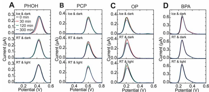
Fig. 1. Baseline corrected square wave voltammograms of 10  $\mu\text{M}$  phenols in pH 12 BR buffer, A) PHOH, B) PCP, C) OP and D) BPA. Stability of different stocks over the time (from 0 till 5 hours) stored in ice and dark; at room temperature (RT) and dark; and at room temperature and daylight.
