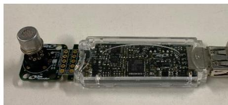
**Figure 1.** JLM MOX STICK device (JLMInnovation GmbH) equipped with a commercial (Figaro TGS2620) sensor.
