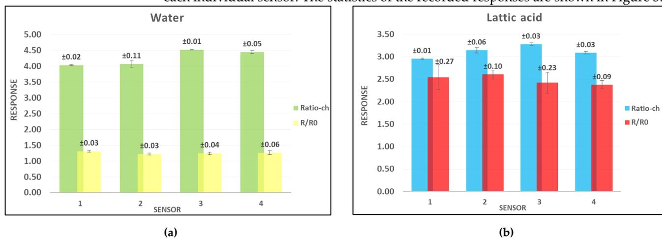
**Figure 3.** (a) Comparison between  $\text{Ratio-CH}$  (green color) and  $R/R_0$  (yellow color) response to water vapors. (b) Response obtained to lactic acid vapors. Light blue rectangles identified  $\text{Ratio-CH}$ , while red rectangles concern  $R/R_0$ .
