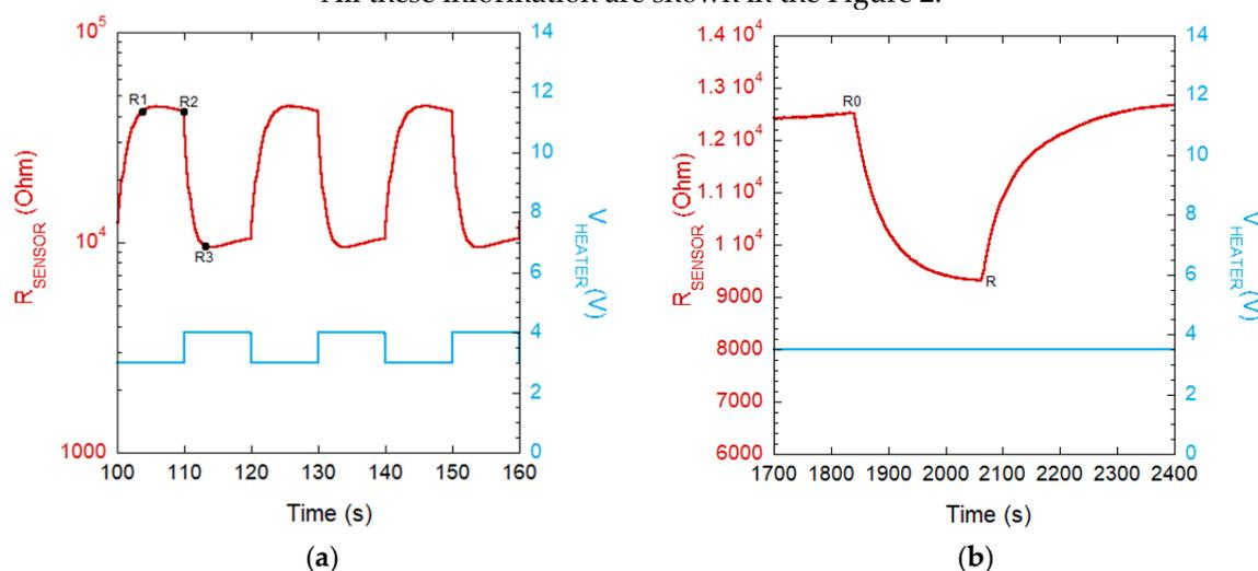
**Figure 2.** (a) The Light blue line represent the modulation of the heater voltage between 3 and 4 volt. The red curve is an example of sensor resistance measured during exposure to water vapors.  $\Delta R-C = R_1 - R_2$ ;  $\text{Ratio-CH} = R_2/R_3$ . (b) The isothermal example showing the voltage applied to the heater with light blue line, while in red curve there is an example sensor resistance measured during exposure to water vapors (response calculated as  $R/R_0$ ).
