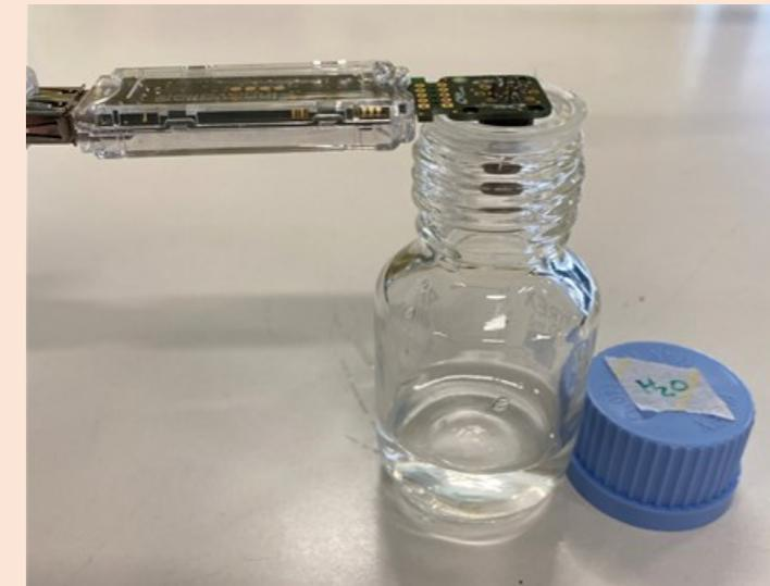
Each sensor was turned on and exposed to ambient air (environmental temperature 21°C) for one hour in order to stabilize before performing the planned series of measurements.
