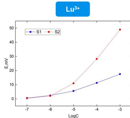
Potentiometric response curve for REMs at pH=2
