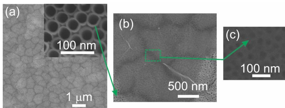
**Figure 1.** SEM images of the obtained samples. (a) The surface morphology of pristine titania nanotubes with different resolutions, (b) and (c) the morphologies of the fabricated composite material with different resolutions.
