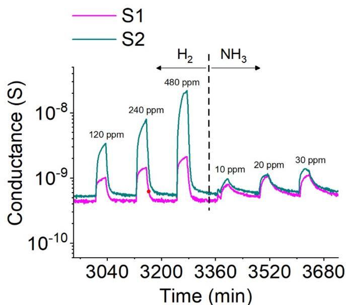
**Figure 2.** The dynamical response of obtained S1 and S2 sensors towards different concentrations of H<sub>2</sub> and NH<sub>3</sub> at 200 °C.
