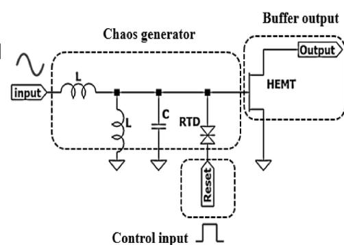
Basic microwave resonant tunneling chaos generator and control circuit
