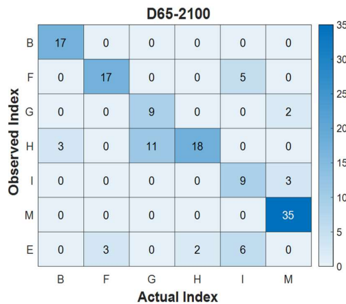
Figure 11. Confusion matrix showing the predictions of superior observers for textile samples under D65 at 2100 lux.
