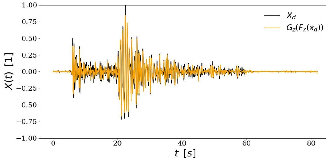
Examples of reconstructed signals for undamaged (top) and damaged (bottom) time-histories. The black lines represent the original time-histories  $x_u^{(i)}$  and  $x_d^{(i)}$  respectively. The orange time histories represent the result of the RepGAN reconstructions  $\mathbf{G}_{\theta_Z} \circ \mathbf{F}_{\theta_X}(x_u^{(i)})$  and  $\mathbf{G}_{\theta_Z} \circ \mathbf{F}_{\theta_X}(x_d^{(i)})$  respectively.
