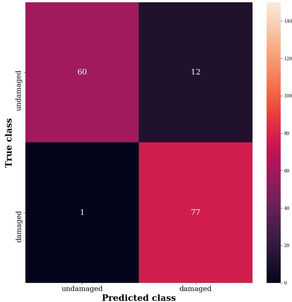
Confusion matrix to further assess the classification accuracy of the model. 60 signals characterized by the undamaged class are correctly classified as undamaged, while only 12 undamaged time histories are identified as damaged. 77 damaged data instances are accurately identified, whereas only one damaged signal is mislabelled.
