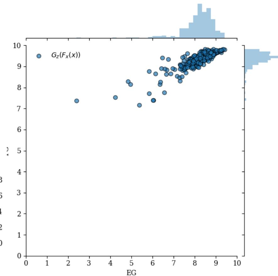
Time-Frequency Goodness-of-Fit (GoF) criterion: evaluation of the fit in Envelope (EG) and the fit in Phase (FG). GoF is evaluated between 0 and 10: the higher the score, the better is the reconstruction.
