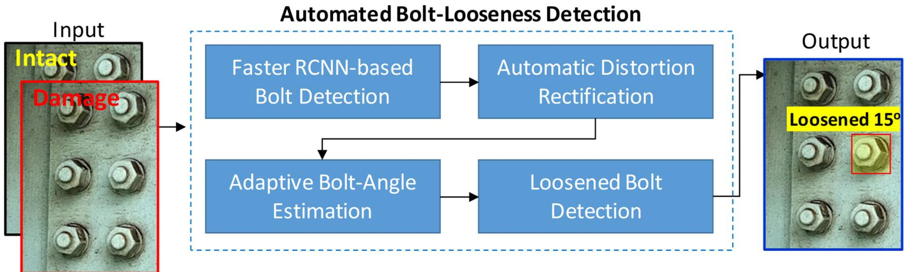
The inputs are the digital images of a bolted connection captured before and after a loosening event and the outputs are the localization of loosened bolts in the images and bolt-looseness degrees. The method is composed of four modules: '*Faster RCNN-based bolt detection*', '*Automatic distortion rectification*', '*Adaptive bolt-angle estimation*', '*Loosened bolt detection*'.
