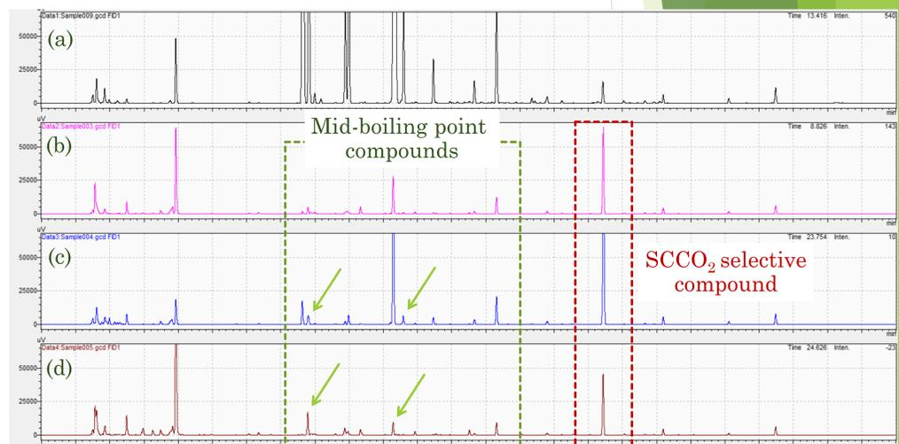
**Figure 2.** The GC chromatograms of black cumin seed oils obtained from (a) screw press machine and SCCO<sub>2</sub> extractions at 20.0 MPa (b) 40 °C, (c) 50 °C, and (d) 60 °C.
