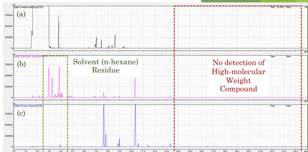
**Figure 1.** The GC chromatograms of (a) n-hexane, (b) Oil obtained from Soxhlet extraction of milled raw seed (Oil<sub>SP</sub>), and (c) the extracted oil obtained from a screw-press machine (Oil<sub>SM</sub>)
