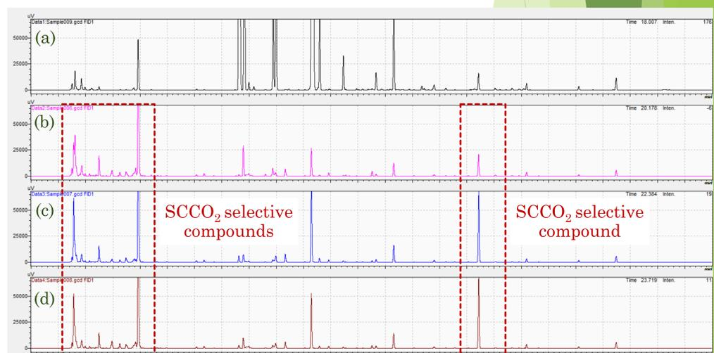
**Figure 3.** The GC chromatograms of black cumin seed oils obtained from (a) screw press machine and SCCO<sub>2</sub> extractions at 30.0 MPa (b) 40 °C, (c) 50 °C, and (d) 60 °C.
