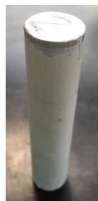
Figure 3. TiO 2 -coated aluminum rod used within the current prototype devices.
