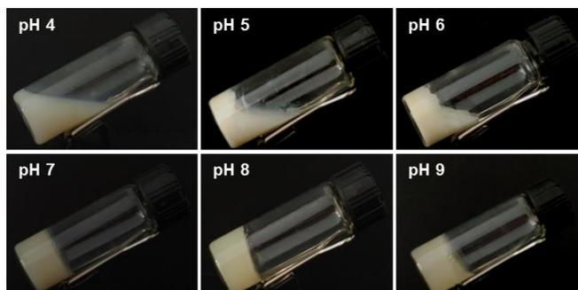
**Figure 2.** The gelation appearance of pcRPIs gels formed at different pH (4–9).
