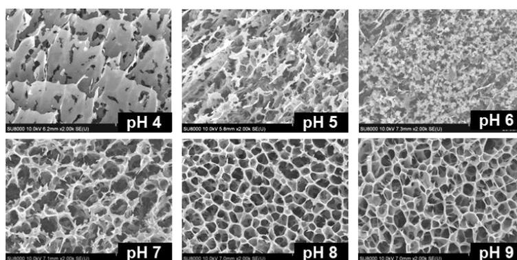
Figure 3. The Cryo-SEM images of pcRPI gels formed at different pH (4 - 9).
