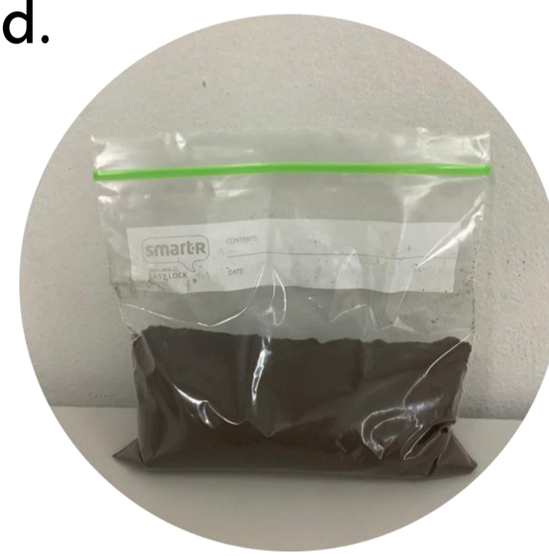
The SCGs sample were dried at 40 °C for 24 hours
