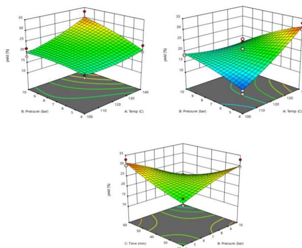
**Figure 1.** (a) Effect of interaction of temperature and pressure and (b) effect of interaction of pressure and time on extraction yield.
