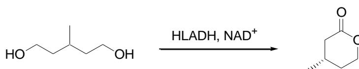
**Scheme 1.** Reaction conditions: [substrate] = [cofactor] = 5 mMn [HLADH] = 0.2 mg/mL, TRIS-HCl or mixtures XoCH/TRIS-HCl, 30 °C, 24 h.
