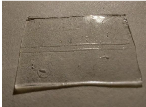
Figure 4. Final fabricated sample. pattern's feature size is 200 micrometers.
