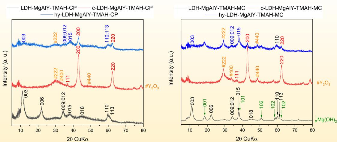
Fig. 1. XRD patterns of samples obtained by co-precipitation method
