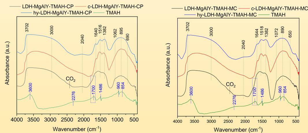
Fig. 3. DRIFT spectra of samples obtained by co-precipitation method
