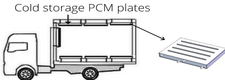
Figure 1. Placement of PCM plates in truck
