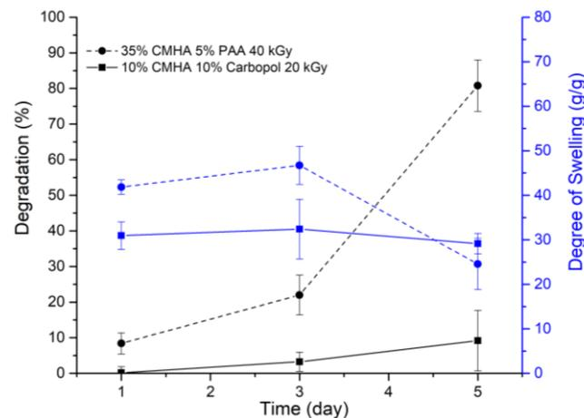
**Figure 5.** In-vitro degradation and swelling property of CMHA with poly(acrylic) acid hydrogels in PBS (pH 7.4) at 37°C
