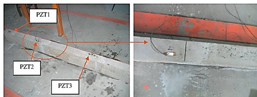
Figure 6. Plain concrete beam with multiple surface-mounted PZT sensors [9].
