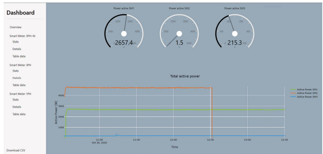
Figure 5. The dashboard's default page. On the right menu, we can select to examine the individual data for each smart meter, while in the middle, we can see the instantaneous values of the active power of the various meters as well as the energy graph.
