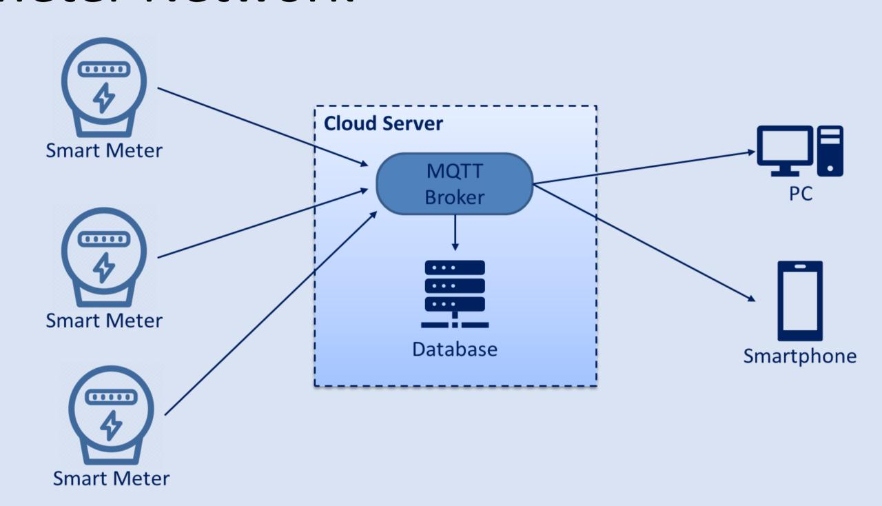
All the smart meters belonging to the network communicate with the cloud through the IoT MQTT protocol.
