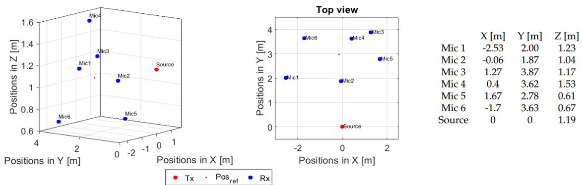
**Figure A1.** Positions of the emitter (E, in red) and the receivers (R, in blue) in the anechoic chamber tests. **(left)** 3D view. **(center)** Top view. **(right)** The Cartesian coordinates
