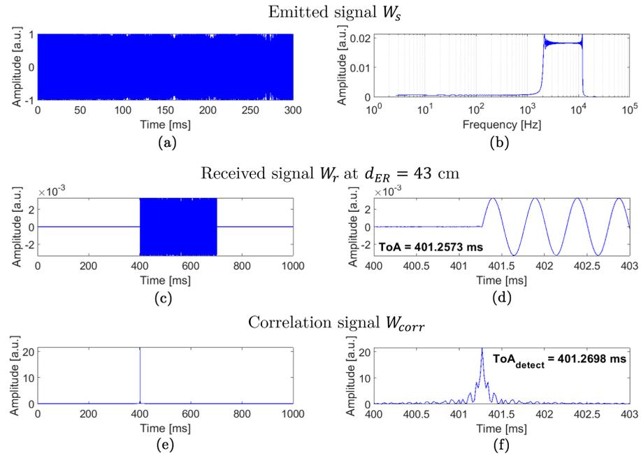
**Figure 1.** (a) Emitted signal in time domain. (b) Emitted signal in frequency domain. (c) Example of received signal (recorded during 1 s) by a receiver placed at a distance of 43 cm from the emitter with a  $ToE$  of 400 ms. (d) Zoom to the  $ToA$  of the received signal. (e) Resulting correlated signal between emitted and received signals. (f) Zoom to the detected  $ToA$  in the correlated signal.
