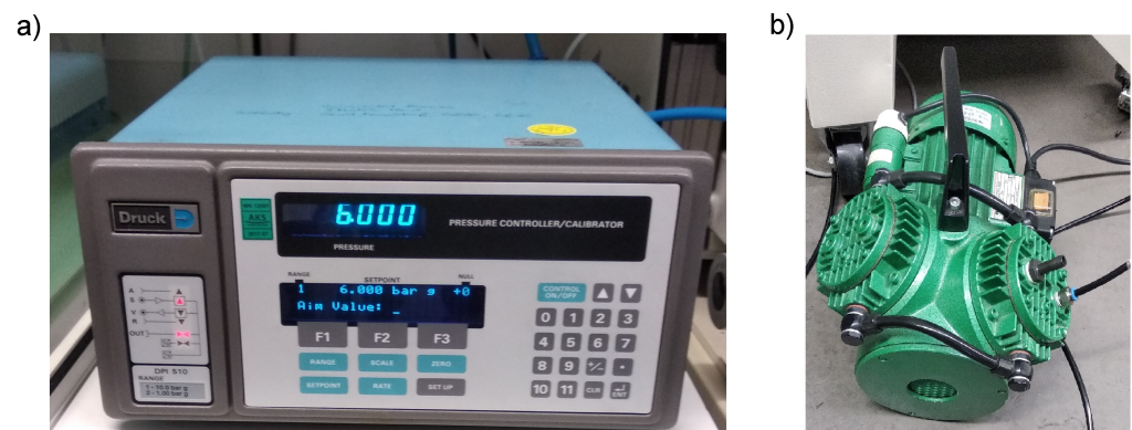
Figure 2. Pressure control equipment. (a) Pressure controller. (b) Vacuum pump.
