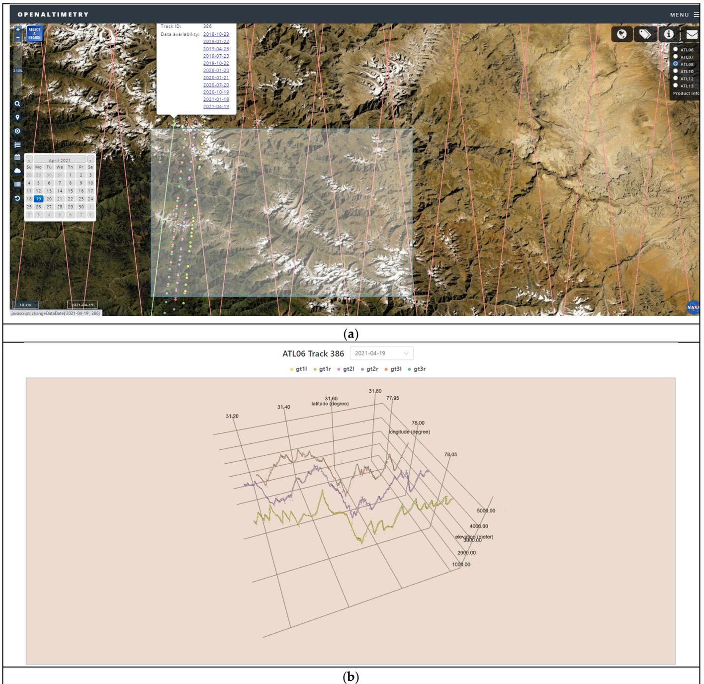
**Figure 2.** Depicts the study area: (a) Parts of Kinnaur District, Himanchal Pradesh and surroundings overlaid with ICESat-2 footprints; (b) Show the OpenAltimetry 3Dviewer describing the terrain cross-sections along the ICESat-2 ground track at footprint/beam locations.
