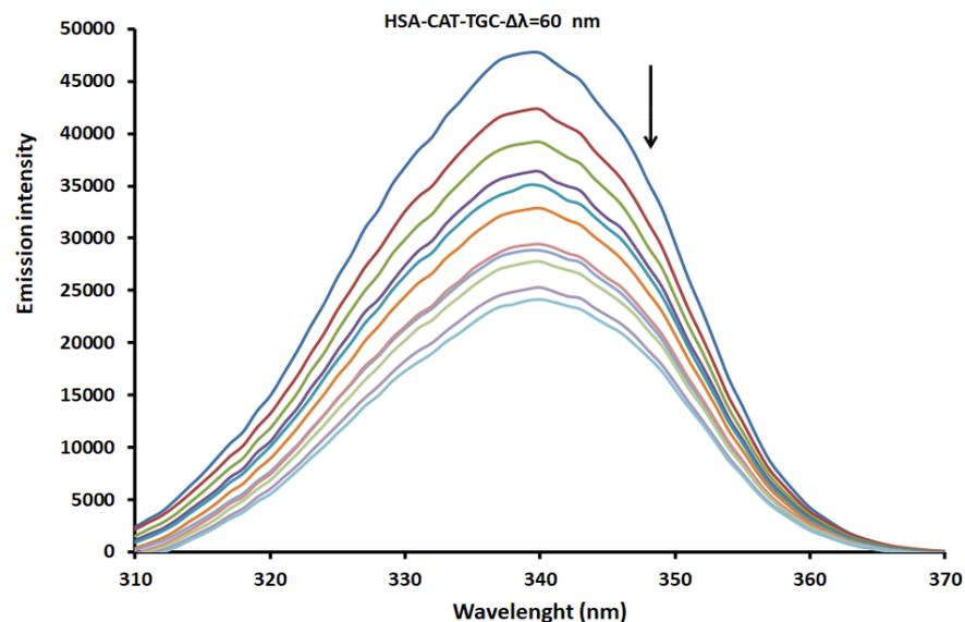
Figure 6. The effect of CAT on the synchronous fluorescence emission spectra of HSA-TGC system (T = 298 K, pH = 7.4). [HSA] = 2  $\mu$ M, [CAT] = 2  $\mu$ M and [TGC] = 0 to 1  $\times 10^{-5}$  M.
