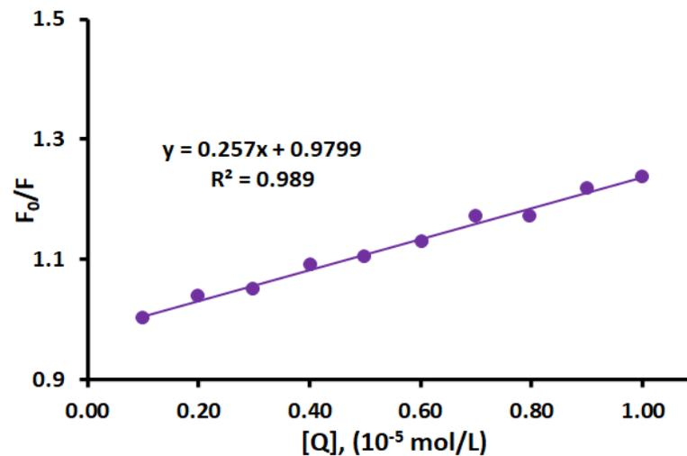
Figure 4. Stern-Volmer plots of the fluorescence quenching of HSA-TGC system by CAT at 298 K<sup>8</sup>
