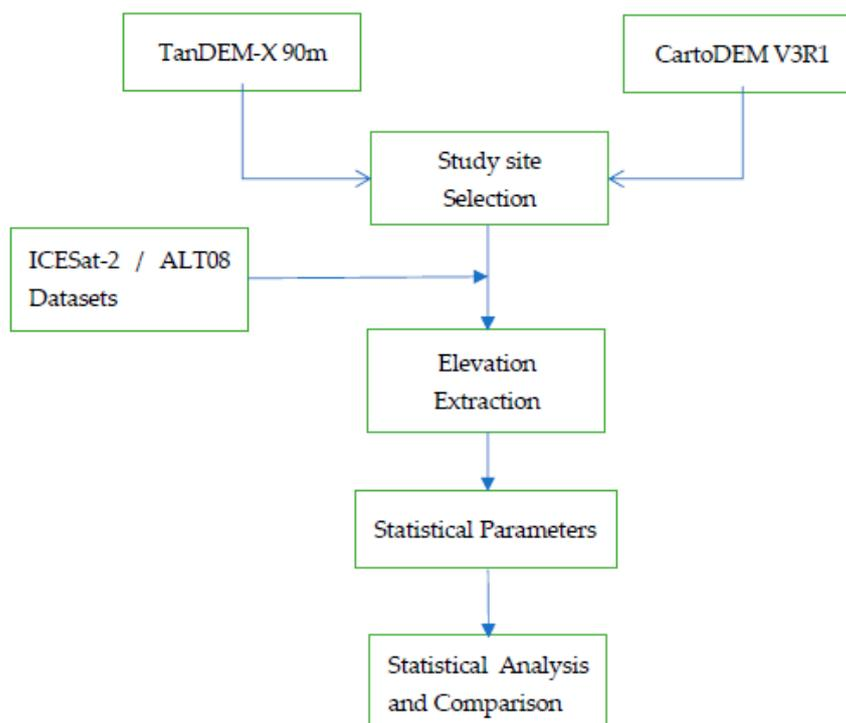
Figure 2. Flow chart of the methodology for DEM evaluation using ICESat-2 datasets
