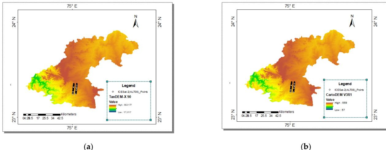
Figure 3. (a) ICESat-2 (ALT08) points superimposed on TanDEM-X 90; (b) ICESat-2 (ALT08) points superimposed on CartoDEM V3 R1.
