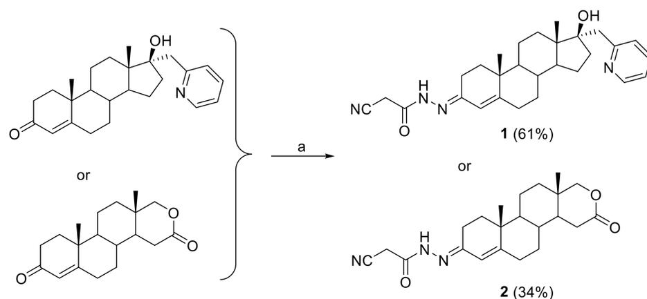
Scheme 1. a) CNCH<sub>2</sub>CONHNH<sub>2</sub>, AcONH<sub>4</sub>, abs. EtOH, reflux, 8h or 13h.
