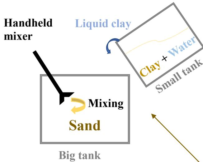
The liquid clay was added into the mixing tank and running the mixer to form a uniformed soil sample. The prepared soil sample was placed in the trench of the flume subsequently.
