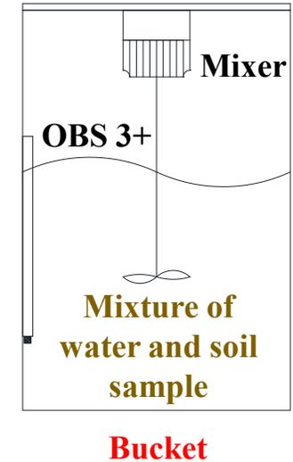
A known quantity of well-mixed dry soil sample was dispersed into the bucket and was suspended in the water by mixer stirring. Meanwhile, OBS signal changes induced by increased SSC were recorded by the connected computer. This process was repeated with known increments of soil sample and the OBS signal were recorded and time-averaged accordingly.
