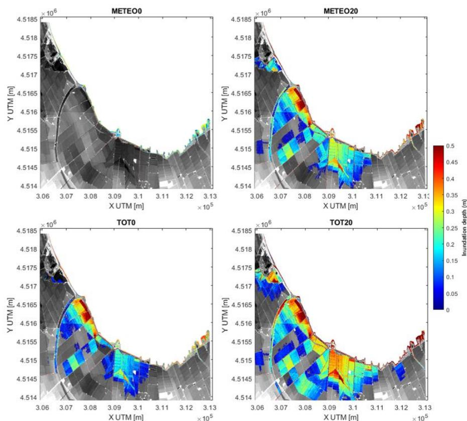
**Figure 3.** Simulation of the inundation of the deltaic plain (only by storm surge) during a Gloria-like storm under current conditions, 0 MSL (left), and + 20 cm MSL (right). Top: only storm-surge component; bottom: total water level (storm surge+astronomical tide).
