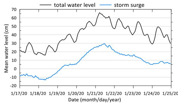
**Figure 2.** Total water level time series recorded during the Gloria storm at Tarragona harbour (data from Puertos del Estado).
