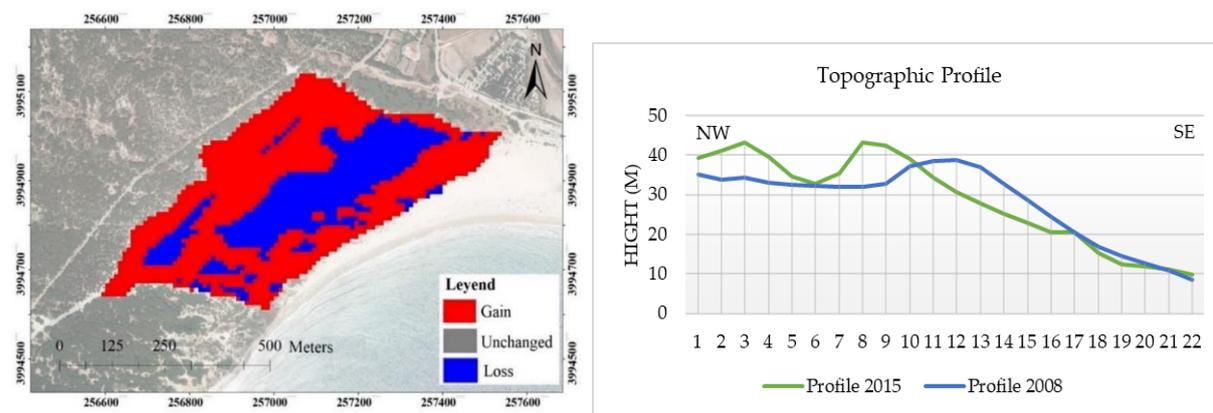
**Figure 2.** Left: Volumetric variation representation of the Valdevaqueros dune, showing loss and gain zones (blue and red) between 2008 and 2015. Right: Topographic Profile of the Valdevaqueros dune for 2008 and 2015.
