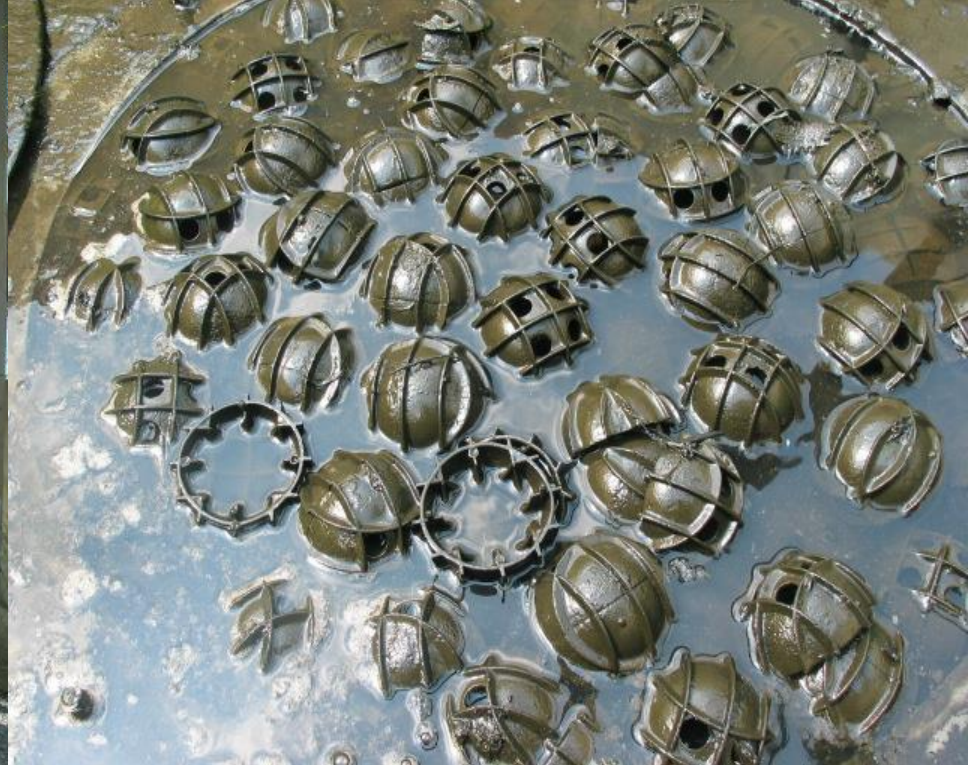
Cosmo-balls media used as supporting biofilm growth
