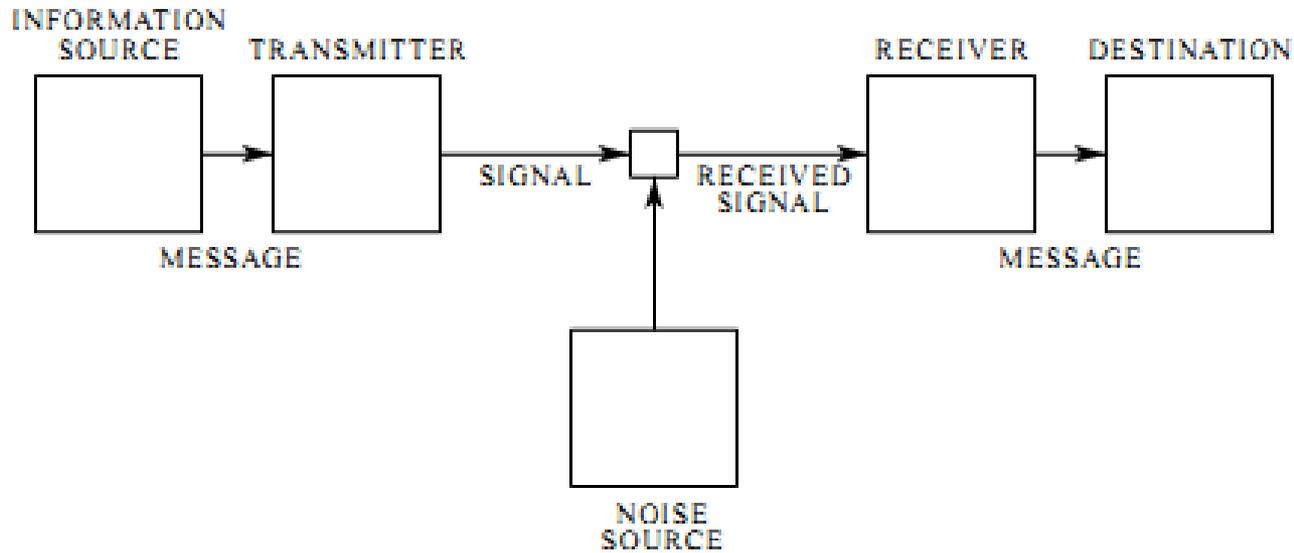
Fig. 1 — Schematic diagram of a general communication system.
