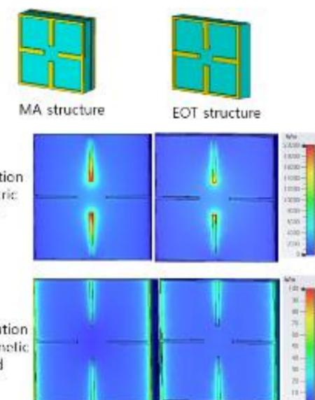
Two spectra very close but the spectrum of transmission broader than that of absorption. The localized electric and magnetic fields on the surface of MA structure seem to be stronger than those of EOT one.
