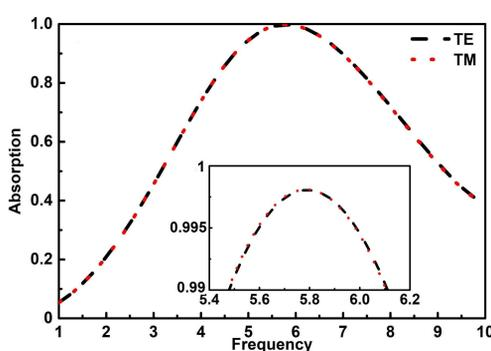
The maximum absorption is 99.8% at 5.79 GHz in the case of TE polarization. Absorption over 99% in a frequency range from 5.48 to 6.1 GHz.
