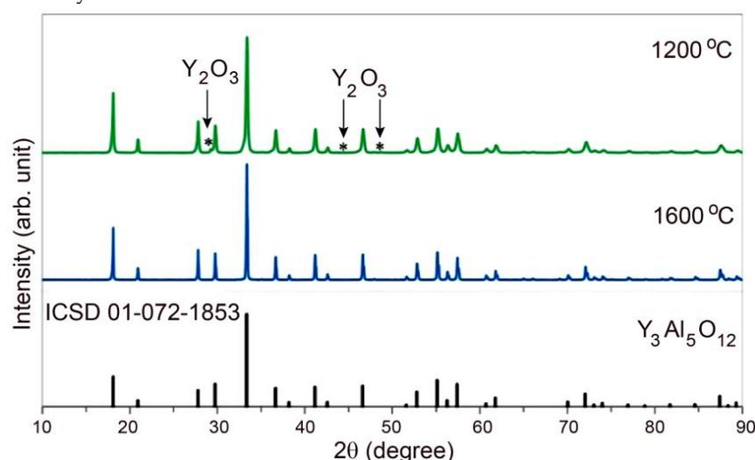
**Figure 1.** X-ray diffraction pattern of the ceramic powder annealed at 1200 °C and 1600 °C in comparison with the XRD pattern of  $Y_3Al_5O_{12}$  from the ICSD database (№ 01-072-1853)
