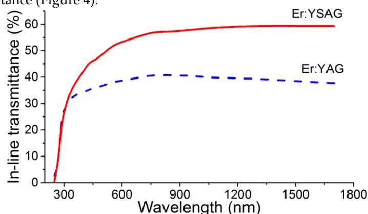
**Figure 4.** In-line transmittance of the  $\text{Er}^{3+}$ :YAG (blue one) and  $\text{Er}^{3+}$ :YSAG (red one) samples
