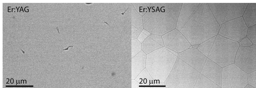
**Figure 3.** SEM micrographs of the Er:YAG and Er:YSAG ceramic surface.
