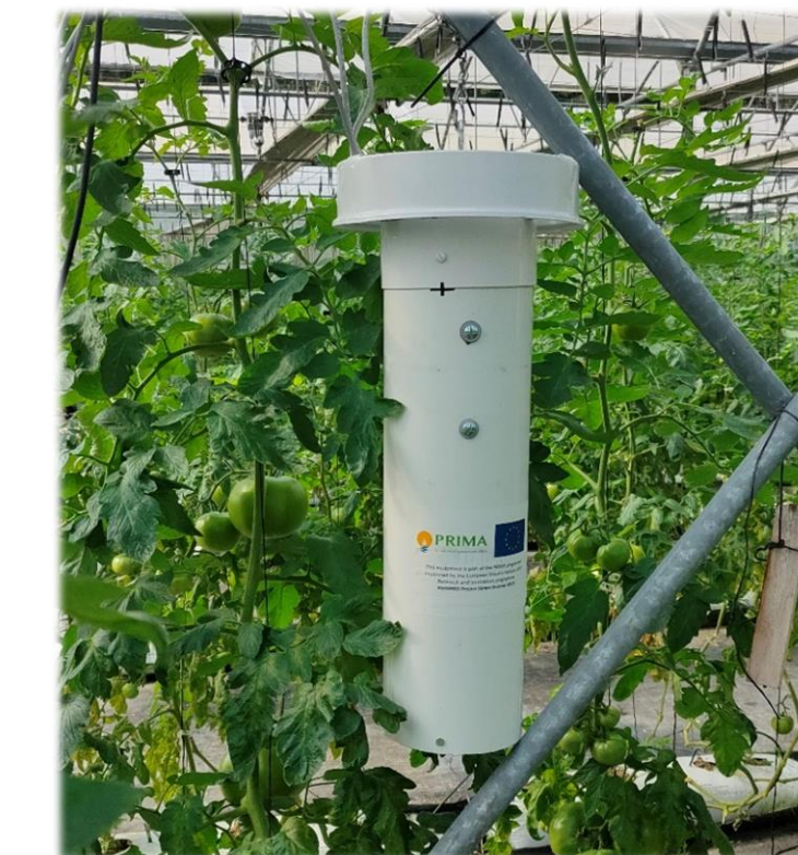
Figure 1: Photograph of the ventilated system used to operate the T and RH sensors.
