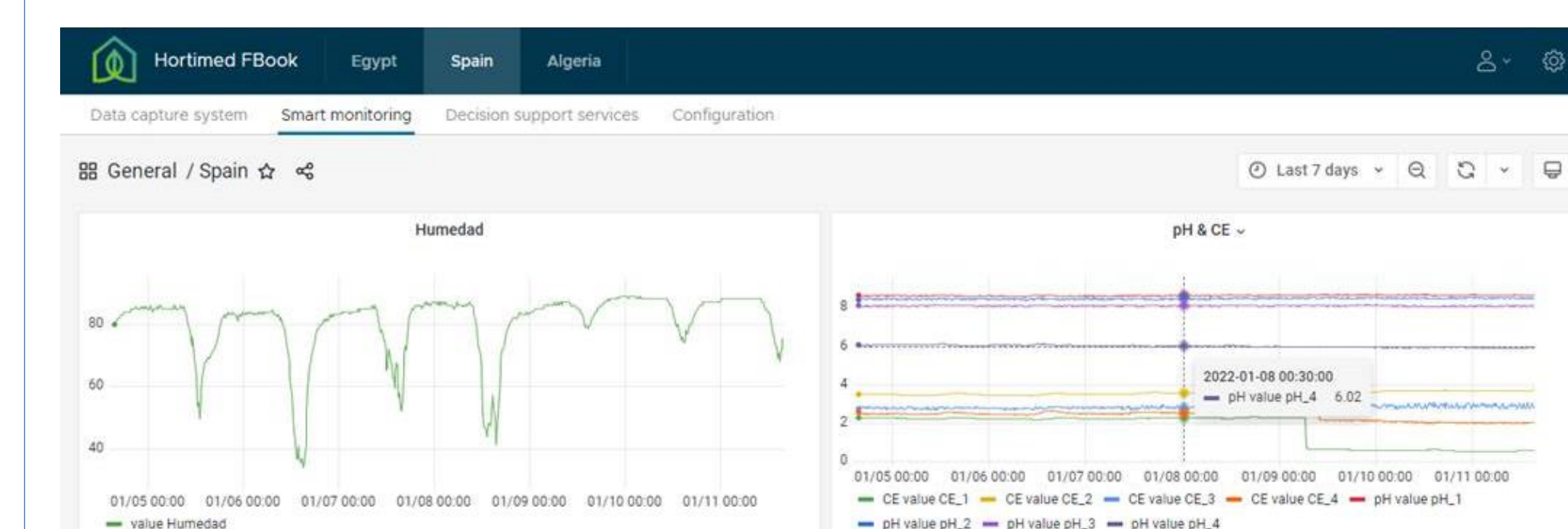
Figure 5: Example illustrating the humidity and pH & CE values measured by the probes located in the HTG (Spain) and automatically transferred to HortiMED's DSS ("Smart Monitoring" section).
