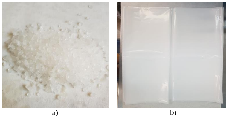
Figure 1. Presentation of a) the pellets of the encapsulated tomato leaves-stem extract in LDPE and b) the final polymeric film with 1% bioactive compounds
