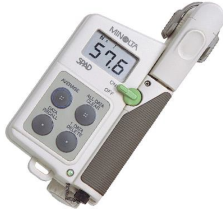
Figure 2: SPAD 502 Plus Chlorophyll Meter (Mohd Firdaus, 2021)
