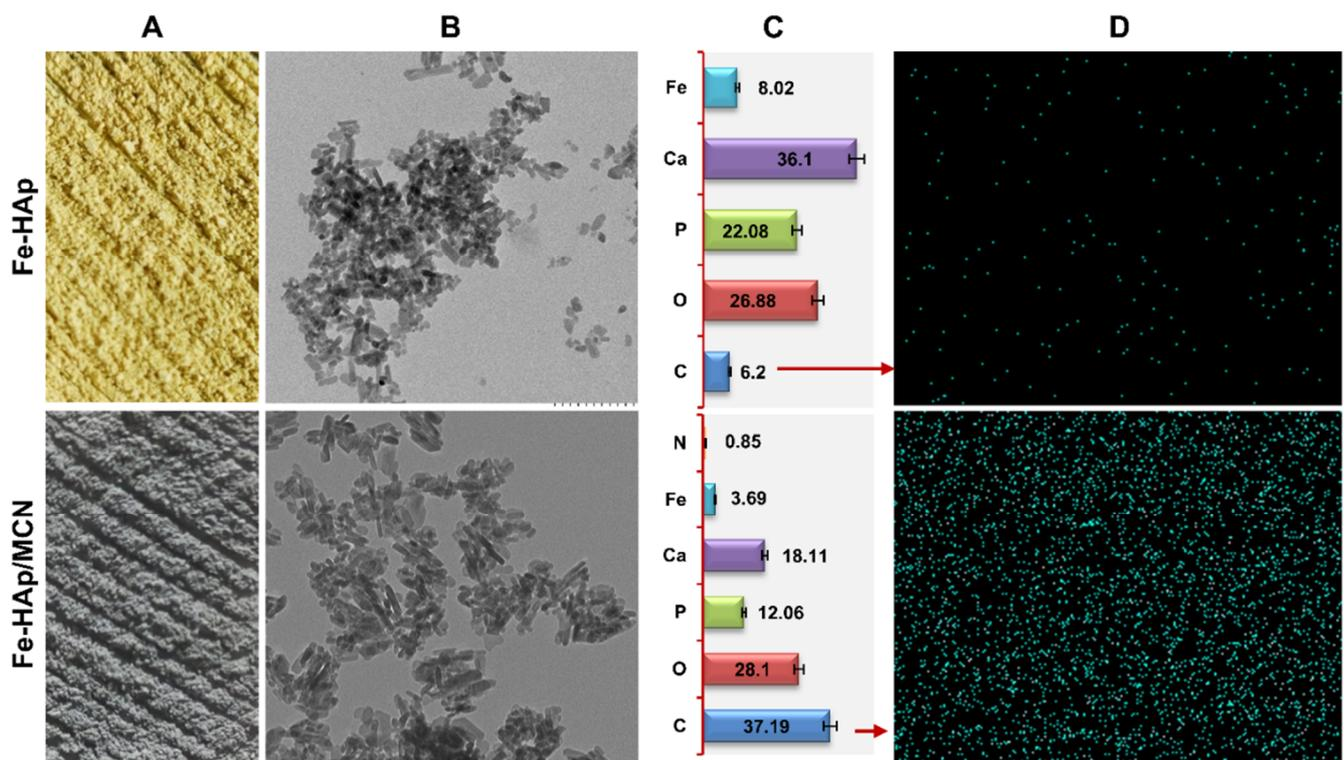
**Figure 1.** (A) Colorimetric morphology of Fe doped HAp nanorods and Fe-HAp/MCN nanorods powder. (B) TEM-based microscopic morphology of Fe doped HAp nanorods and Fe-HAp/MCN nanorods. Scale bar, 200 nm. (C) The EDS-based atomic percentage of various elements present in Fe doped HAp nanorods and Fe-HAp/MCN nanorods. (D) EDS mapping of elements present in Fe-HAp nanorods and Fe-HAp/MCN nanorods.
