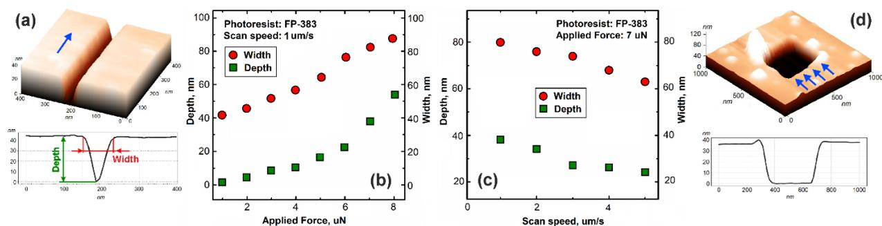
**Figure 1.** Study of scratching probe nanolithography modes on FP-383 photoresist: 3D-AFM image and AFM cross section of a single nanostructure (a); Dependencies of the photoresist puncture depth and structure width on the applied force (b) and scan speed (c); 3D-AFM image and AFM cross section of a complex nanostructure (d).
