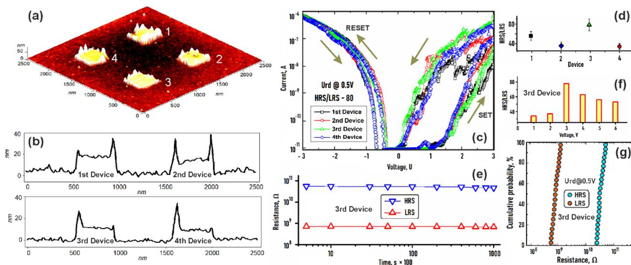
**Figure 2.** Resistive switching of the TiN/ZnO/TiN/Al<sub>2</sub>O<sub>3</sub> structure (4 devices): (a)–3D AFM image of the ZnO film and TiN electrodes; (b)–AFM cross-section; (c)–current-voltage characteristics; (d)–HRS/LRS ratio; (e)–retention test; (f)–HRS/LRS ratio dependence on the amplitude of the CVC pulse ( $U_{rd} = 0.5$  V); (g)–cumulative probability.
