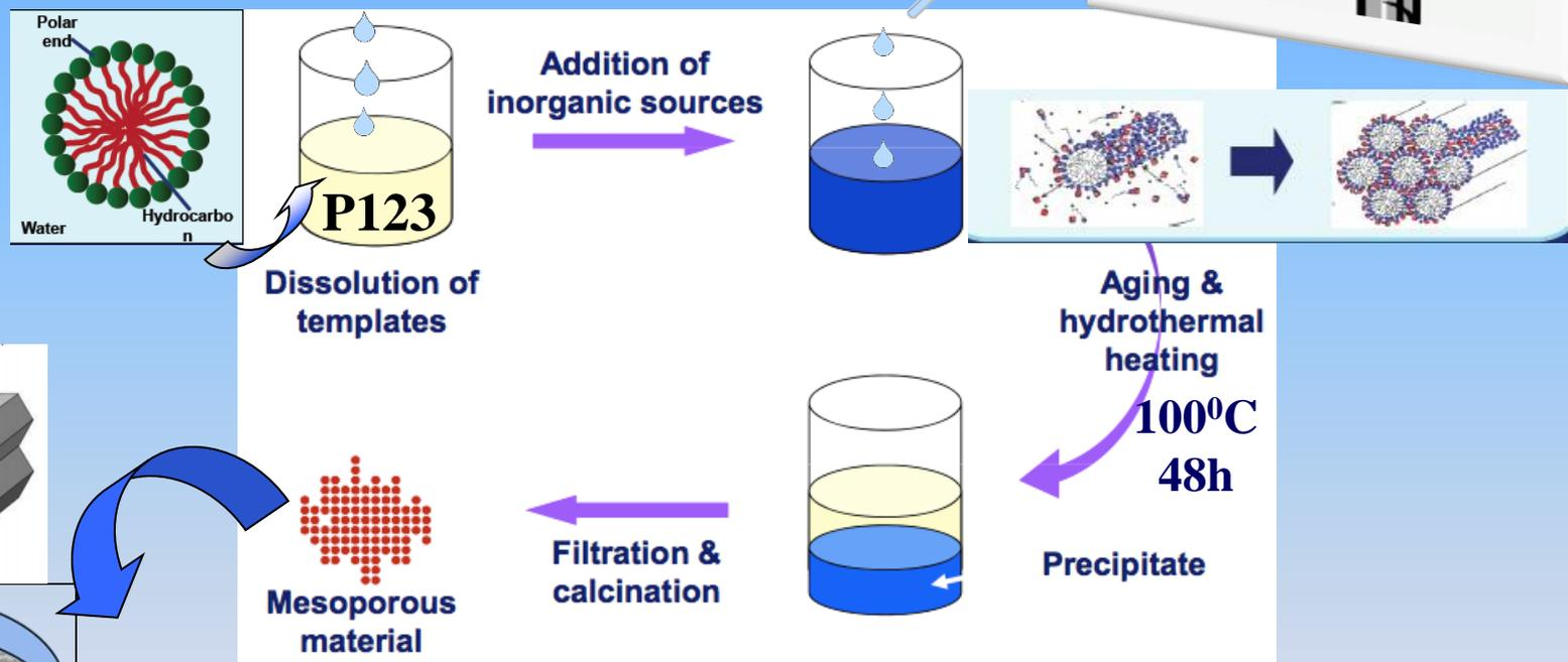
•The obtained solids were further used as supports for impregnation, by incipient wetness technique, with an aqueous solution of platinum ( $H_2PtCl_6$ ) and cerium  $Ce(NO_3)_3$  in order to prepare catalysts with 0.25, 0.5, and 1% Pt, respectively, 1%  $CeO_2$ .
