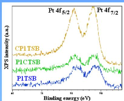
XPS spectra of Pt and Ce modified mesoporous silica
