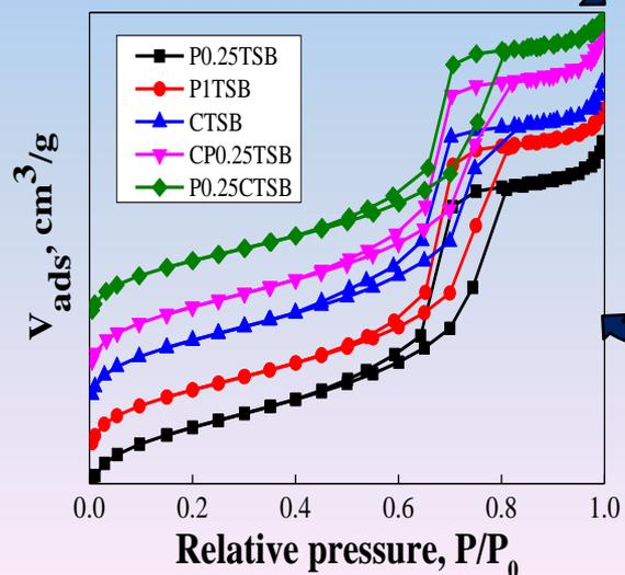
N<sub>2</sub> adsorption-desorption isotherms and pore size distribution
