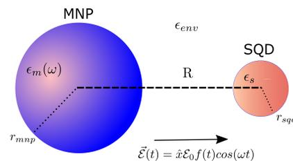
**Figure 1.** Semiconductor quantum dot-metal nanoparticle coupled systems.
