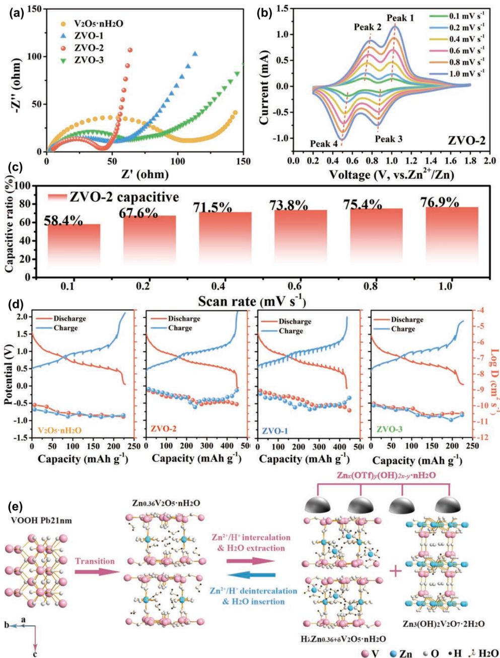
Fig 3. EIS patterns of all samples (a), CV profiles of ZVO-2 at different scan rates (b), the contribution ratio of capacitive capacities in ZVO-2. (c), GITT profiles and diffusion coefficients of all samples (d), Schematic diagram of the  $Zn^{2+}/H^+$  insertion mechanism on ZVO-2 cathode (e).
