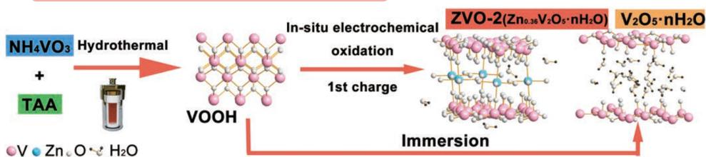
Scheme 1. Schematic diagram of preparation of VOOH and conversion from VOOH to ZVO and  $V_2O_5 \cdot nH_2O$ .
