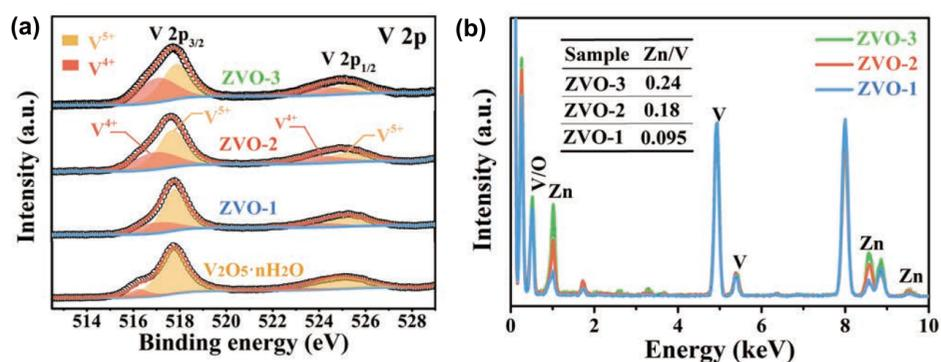
Fig 1. V 2p spectra of ZVO and  $V_2O_5 \cdot nH_2O$  (a) and EDS spectra of ZVO (b).
