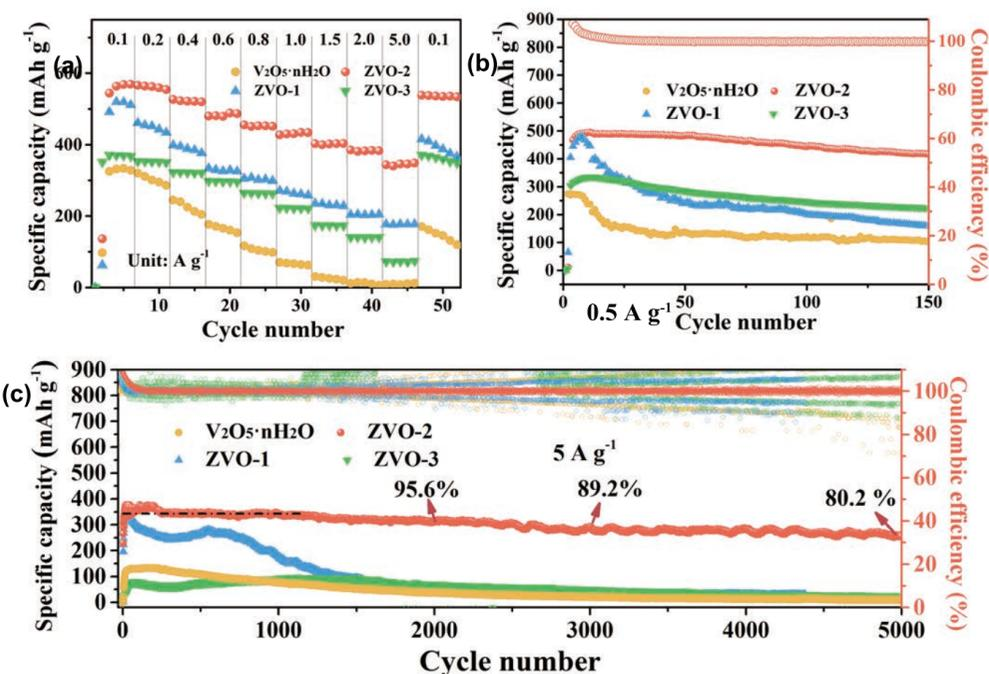
Fig 2. Electrochemical properties of ZVO and  $V_2O_5 \cdot nH_2O$  (electrochemical chain: Zn foil|3 M  $Zn(OTf)_2$ |ZVO or  $V_2O_5 \cdot nH_2O$ ). (a) Rate performance of ZVO and  $V_2O_5 \cdot nH_2O$ . (b) Cyclability of ZVO and  $V_2O_5 \cdot nH_2O$  at  $0.5 A g^{-1}$ . (c) Cyclability of ZVO and  $V_2O_5 \cdot nH_2O$  at  $5 A g^{-1}$ .
