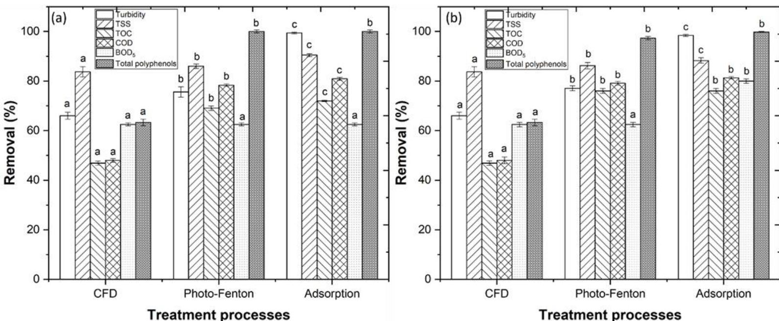
Removal efficiency of (a) CFD/UV-A-Fenton/Adsorption system, (b) CFD/UV-C-Fenton/Adsorption system. CFD operational conditions: [PVPP] = 0.5 g/L, pH = 6.0, rapid mix (rpm/min) = 150/3, slow mix (rpm/min) = 20/20, sedimentation = 12 h. Photo-Fenton operational conditions: [Fe<sup>2+</sup>] = 2.5 mM, [H<sub>2</sub>O<sub>2</sub>] = 225 mM, pH = 3.0, agitation = 350 rpm, t = 150 min. Adsorption operational conditions: [Bentonite] = 1.5 g/L, pH = 6.0, agitation = 350 rpm, sedimentation = 2 h.
