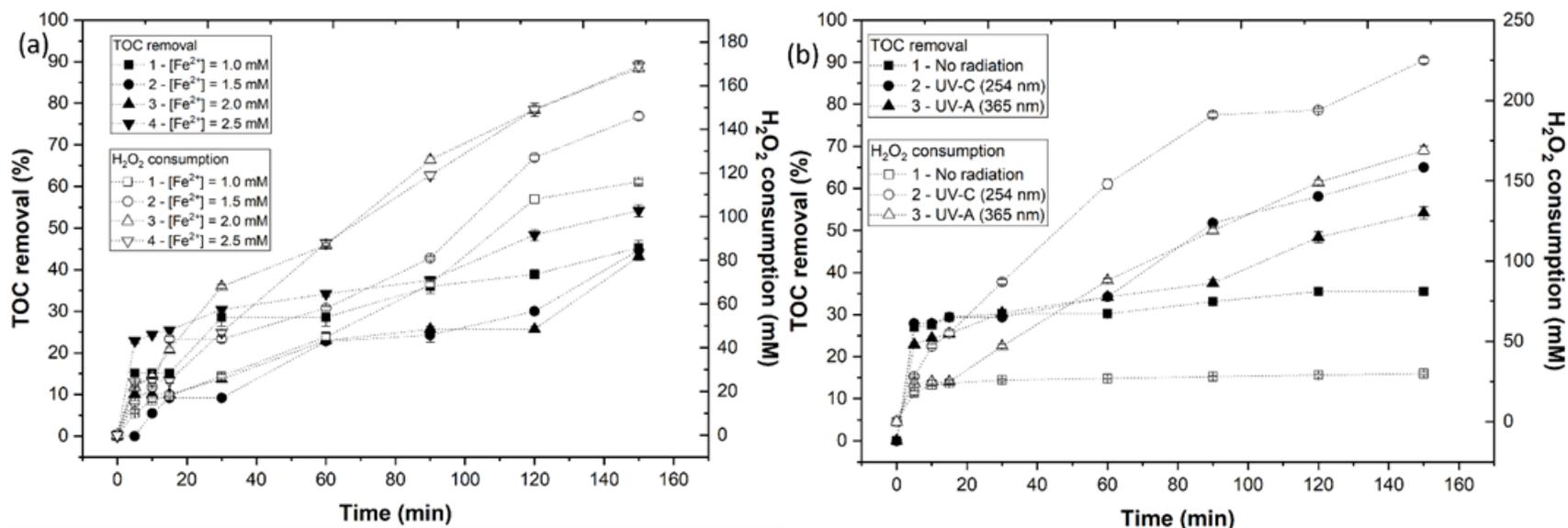
(a) TOC and H<sub>2</sub>O<sub>2</sub> consumption with Fe<sup>2+</sup> variation (1.0 – 2.5 mM) under operational conditions: pH = 3.0, radiation = UV-A IUUV = 32.7 W/m<sup>2</sup>, agitation = 350 rpm, t = 150 min; (b) TOC and H<sub>2</sub>O<sub>2</sub> consumption with radiation type variation (no radiation, UV-C and UV-A) under operational conditions: [Fe<sup>2+</sup>] = 2.5 mM, pH = 3.0, agitation = 350 rpm, t = 150 min.
