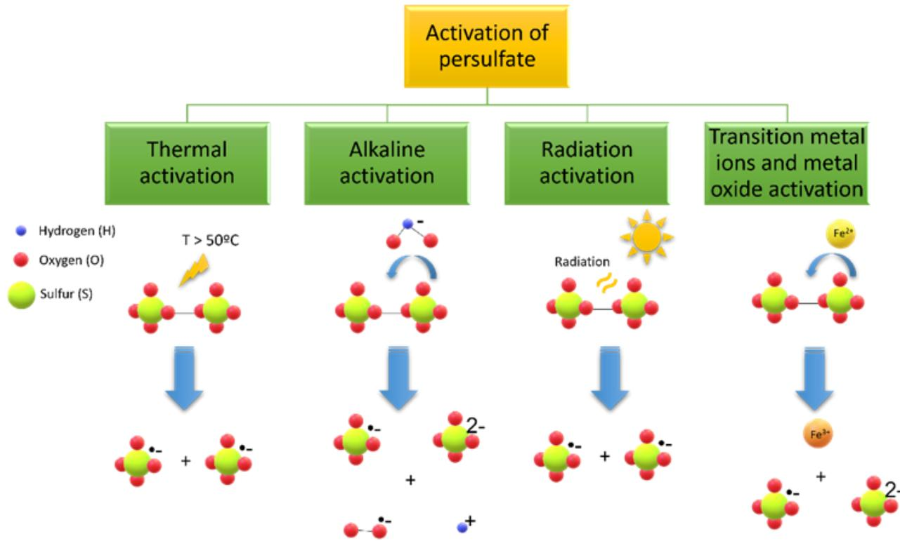
Schematic representation of the activation mechanism of persulfate.
