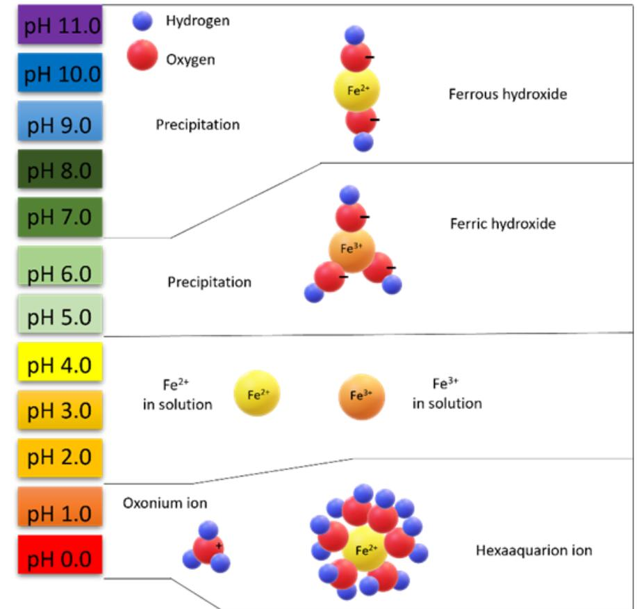
Precipitation and form of iron catalyst at different pH.
