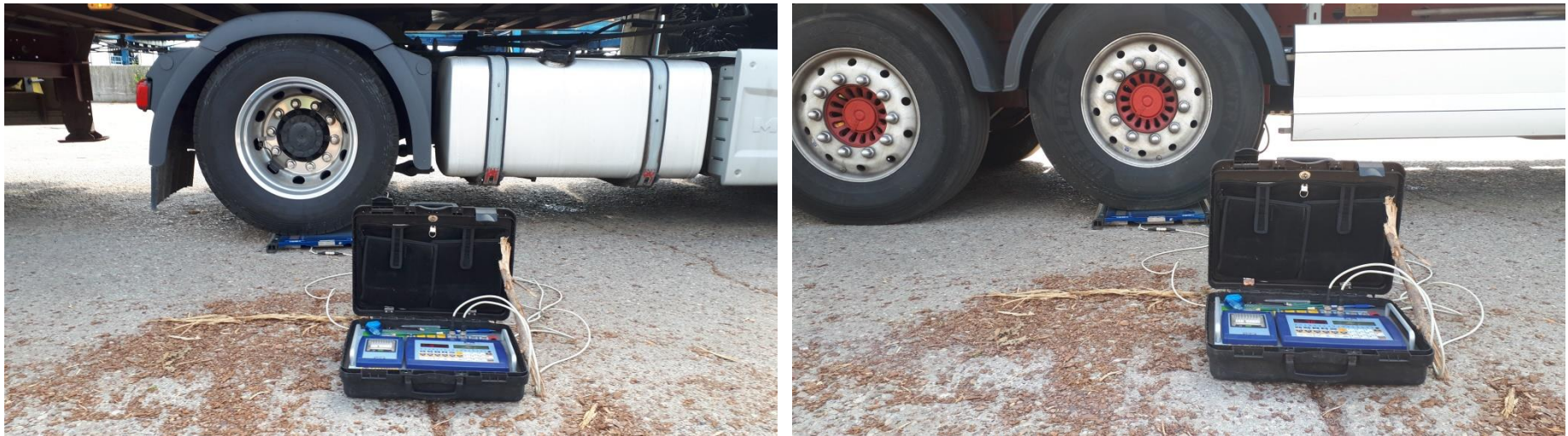
Figure 2. Measured the load on the individual axles of high tonnage truck units. Weighing the wheel axles of a truck unit hauling timber.
