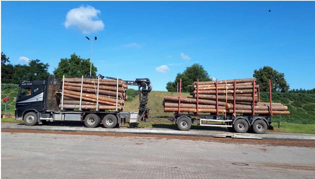
Figure 1. Weighing station for whole transport sets on a stationary scale (roundwood carried by truck and trailer).
